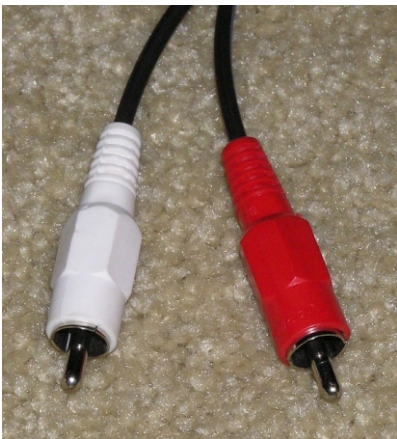
RCA Audio Stereo Left (white) and Right (red)
