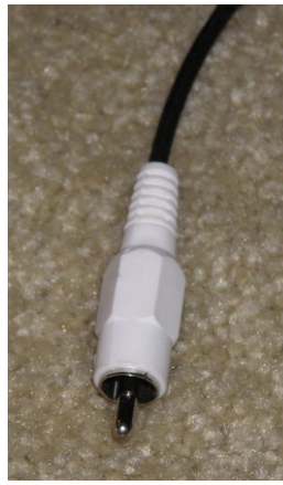
RCA Audio Single (use in Left if 2 jacks)
