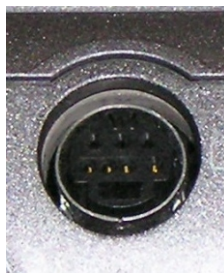
S-Video Cable and Port (Better video than RCA)
