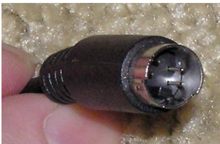
S-Video Cable and Port (Better video than RCA)
