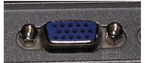
VGA port on Computer, AverKey, or Projector
